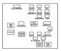
The instrument panel fuse block is located on the passenger's side of the instrument panel.
